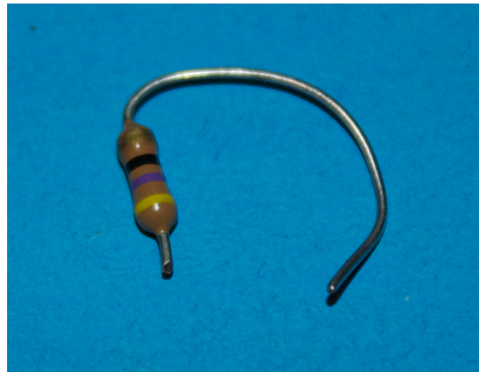
Figure 4 – A suitable axial-lead resistor. This one is 47 ohms, 1/4 watt.
